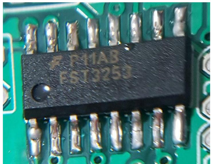
necessary, you can remove solder bridges with desoldering braid.
