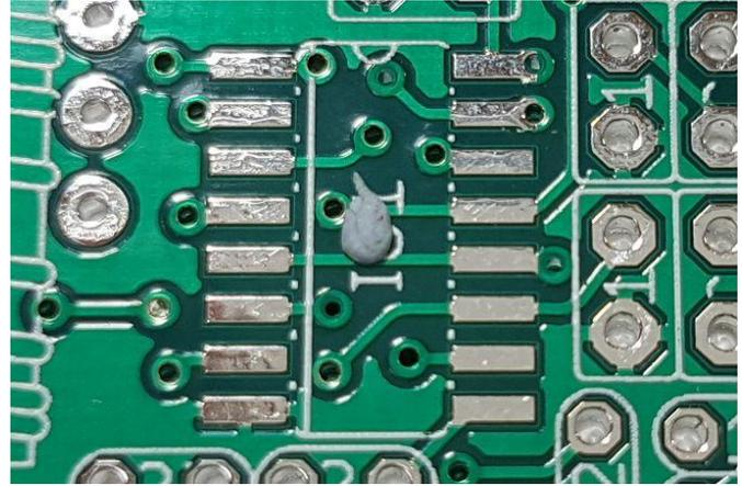
Check the pins of the FST3253 and if any are bent, straighten them carefully and very gently. Place the IC on the PCB with the small dimple aligned with the mark on the PCB. It is very important to orientate this IC correctly. You can check the alignment of each pin against its PCB pad using a jeweller's loupe or magnifying glass. (below left).
