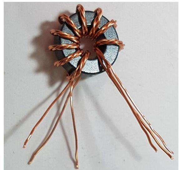
Now it's necessary to identify which wire belongs to which winding. You have three windings twisted together, they all use the same wire. The only way to do this is with a DVM as continuity tester. First, untwist and straighten the wire ends that are not wound around the toroidal core.
