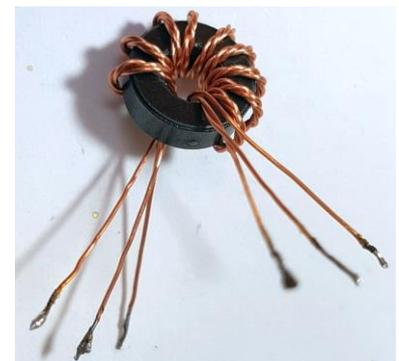
Now use a DVM to test for continuity. Re-arrange the wires so that there is continuity from A-A, B-B, and C-C in this photo.
