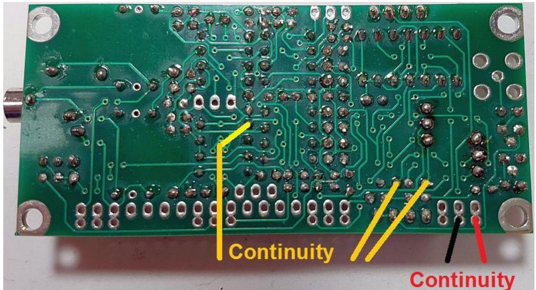
Next check for continuity between pin 1 of IC6 and the ends of the two 82-ohm resistors R26 and R27. Hold the black probe on IC6 pin 1. Hold the red probe on the resistor ends as indicated by the two nearby orange lines.
