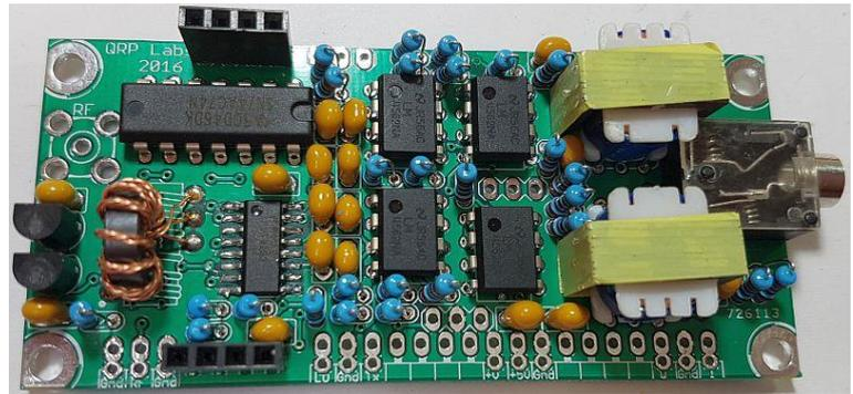
Try to fit the toroid as far left as possible, as in this photo, so that it does not interfere with the Band Pass Filter module when plugged in.
